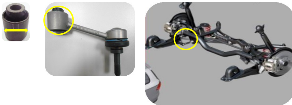
Fig. 1. Rubber bushing with mold bonded metal sleeves
