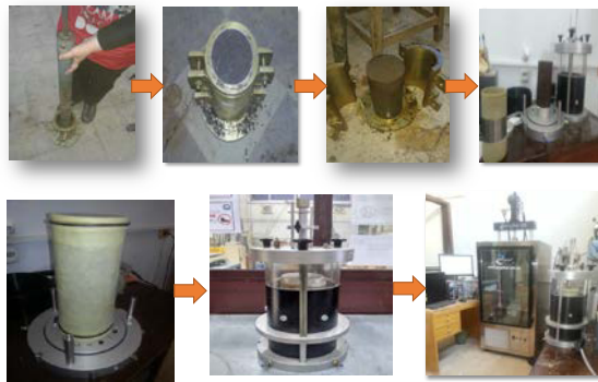
Fig. 2. Sample preparation and test set up.
