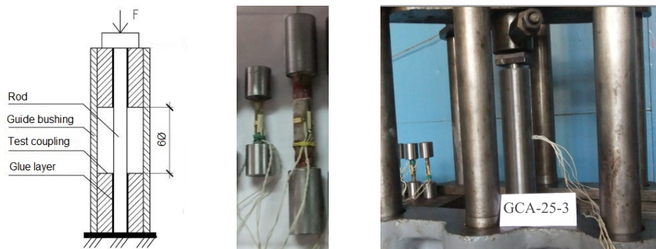
Fig. 1. Schemes of testing composite samples for axial compression
