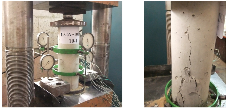
Fig. 6. General view of tests and destruction nature of concrete samples (series CCA) with glass composite reinforcement under compression
