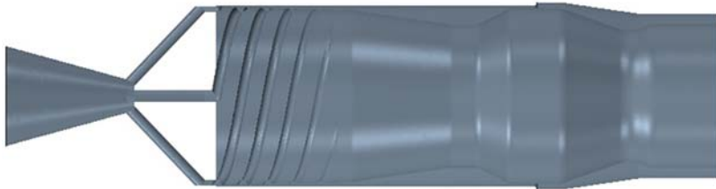
Fig. 5. Volume of raw material inside the head with four inputs.
