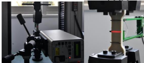
**Figure 1.** Tensile test and strain measurement experiment
