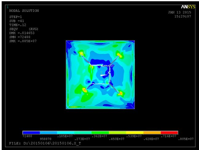
Figure 6. The stress distribution of the moment of cracking
