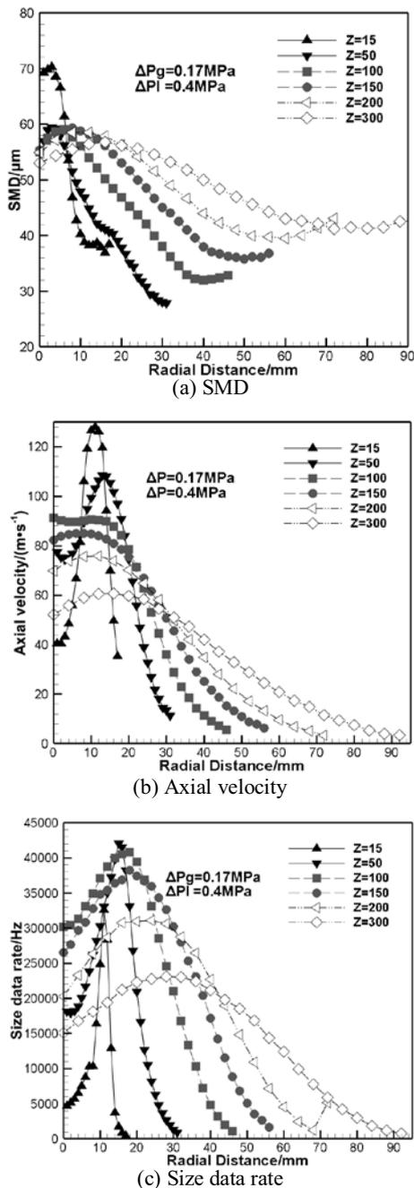
Figure 5. Spatial distribution of gas-liquid coaxial swirl injector.
