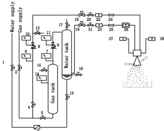
Figure 2. Test system schematic diagram.
