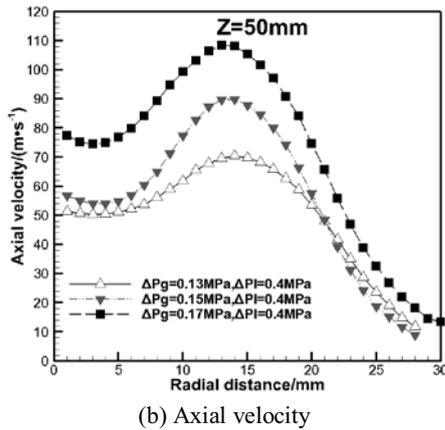
**Figure 7.** Spatial profiles of SMD and axial velocity under different gas pressure drop.
