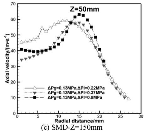
**Figure 8.** Spatial profiles of SMD and axial velocity under different liquid pressure drop.
