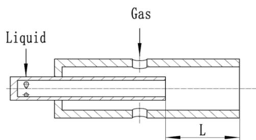
**Figure 1.** Schematic of gas-liquid coaxial swirl injector.
