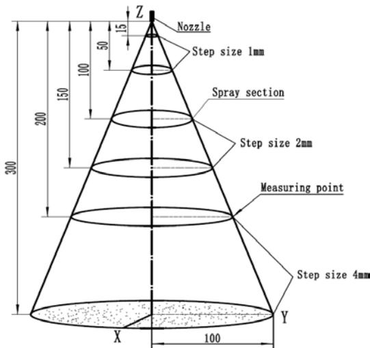
Figure 3. Measuring planes and points.
