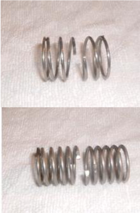
Figure 2. Fractured spring of suction liquid valve and discharge liquid valve
