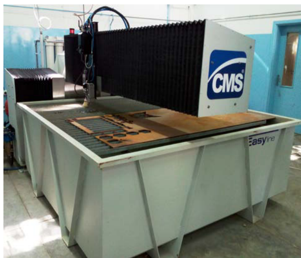
Figure 1. Abrasive water jet machine type (CMS EASYLINE 7785).
