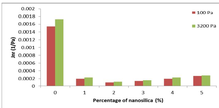
**Fig. 4.** Nonrecoverable creep compliance ( $J_{nr}$ ) at difference stress level of NSMB
