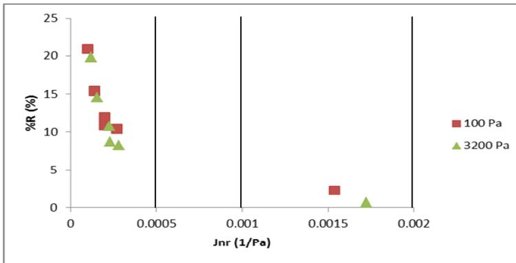
**Fig. 7.** Relationship between J<sub>nr</sub> and %R of NSMB
