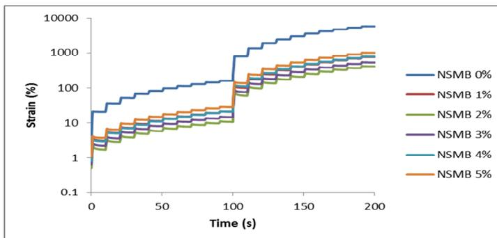
Fig. 2. Strain versus time of MSCR testing for ten cycle
