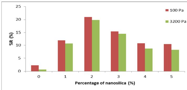
Fig. 5. Percent recoverable strain (%R) at difference stress level of NSMB
