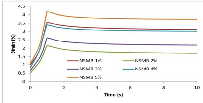
**Fig. 3.** Strain versus time of MSCR testing for one cycle at 100 Pa
