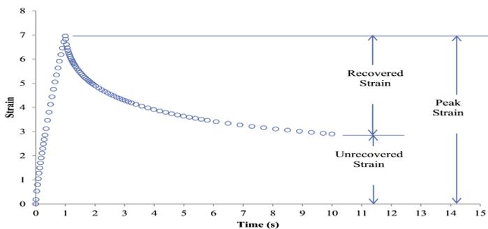
**Fig. 1.** Typical creep and recovery in MSCR test
