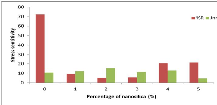
**Fig. 6.** Stress sensitivity of %R and J<sub>nr</sub> of NSMB
