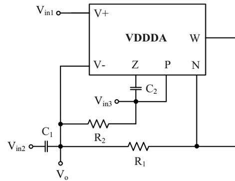
**Figure 2.** VDDDA based voltage mode TISO filter.
