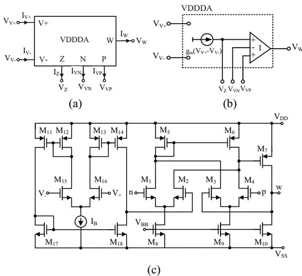
**Figure 1.** VDDDA, (a) circuit symbol, (b) equivalent circuit and (c) schematic diagram of CMOS VDDDA
