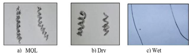
Figure 3. Chips produced under MQL, Dry and Wet under same parameters.
