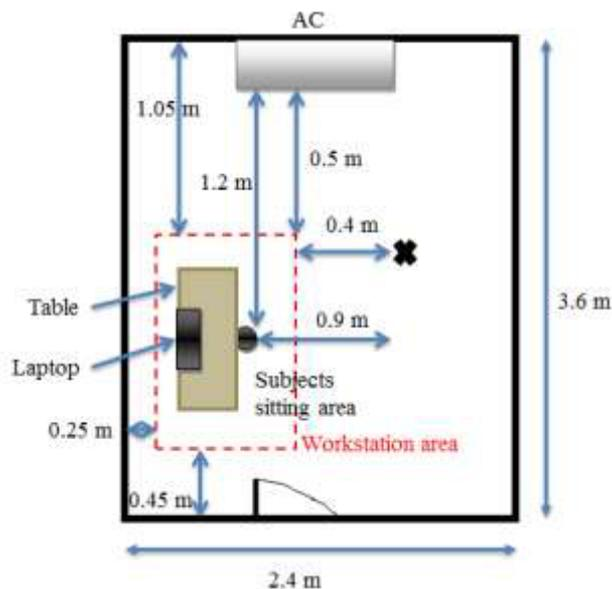
**Fig. 1.** The arrangement in environmental chamber.
