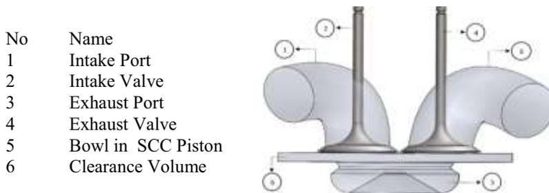
**Fig. 3.** Engine components.
