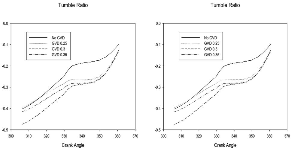
**Fig. 6.** (a) Tumble ratio against crank angle ( $\theta$ ) and (b) Cross tumble ratio against crank angle ( $\theta$ ).
