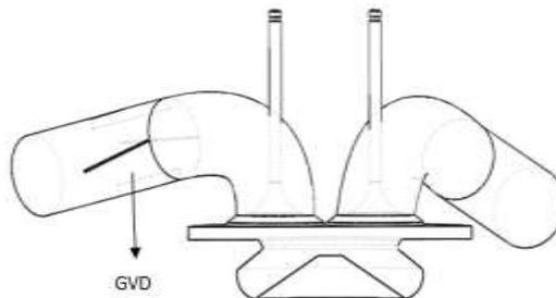
**Fig. 4.** GVD installation at the intake manifold.
