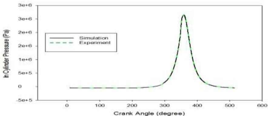
**Fig. 2.** In-cylinder pressure against crank angle ( $\theta$ ).
