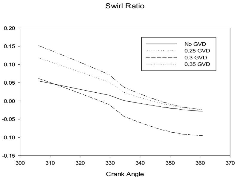
**Fig. 5.** Swirl ratio against crank angle ( $\theta$ ) with and without GVD.
