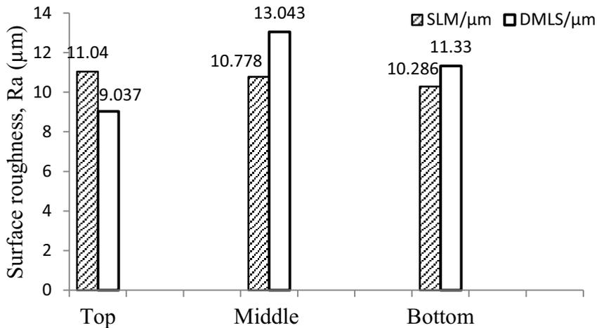
Fig. 5. Comparison surface roughness ICCT of different process.
