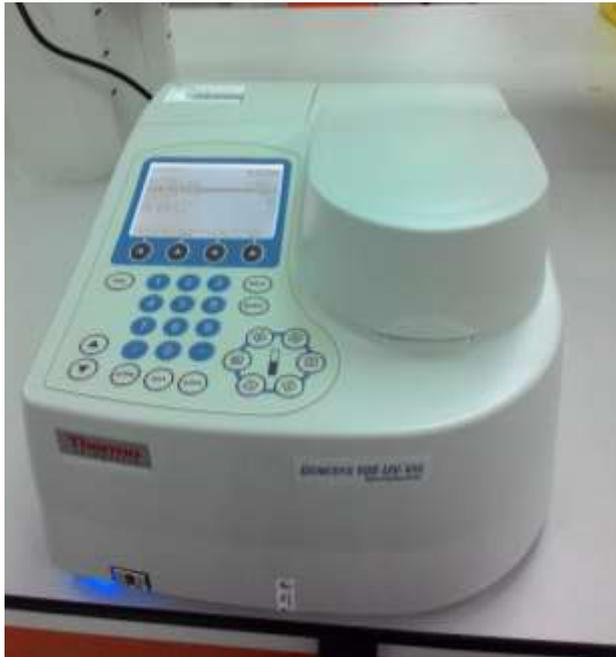
**Fig. 2.** Genesys 10 UV-Vis Spectrometer.
