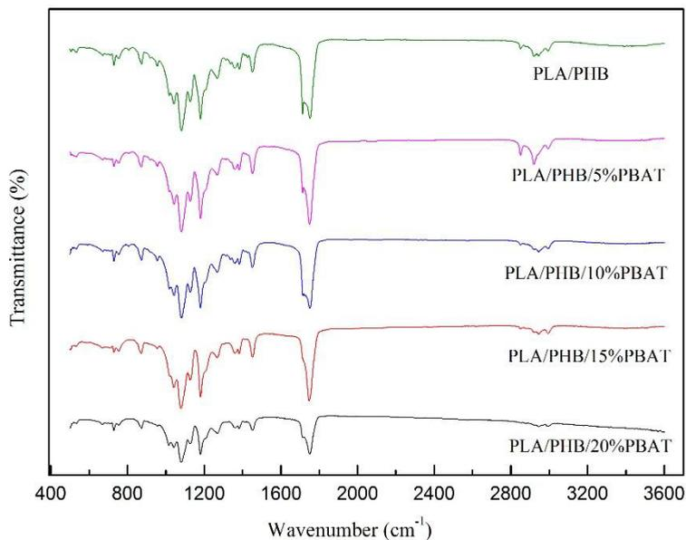
**Figure 2.** FT-IR spectra of PLA/PHB and PLA/PHB/PBAT samples in 400cm<sup>-1</sup>~3600cm<sup>-1</sup>.
