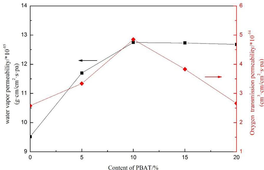
**Figure 1.** Effect of PBAT on oxygen and water vapor permeability of film
