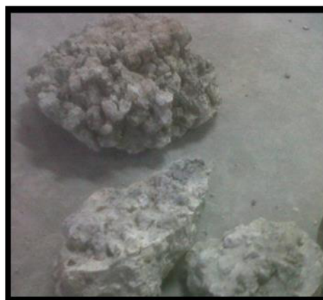
Figure 1. (a) RCA samples from CDW
