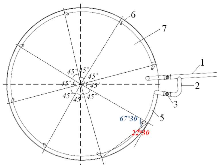
**Fig. 3.** Design of funnel type cleaning system for sludge removal.
