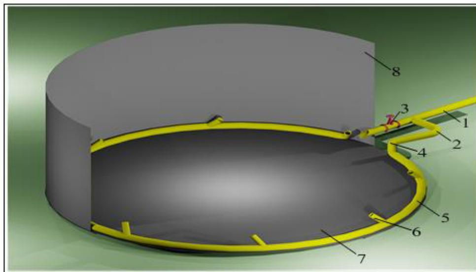
**Fig. 2.** General view of funnel type cleaning system for sludge removal.
