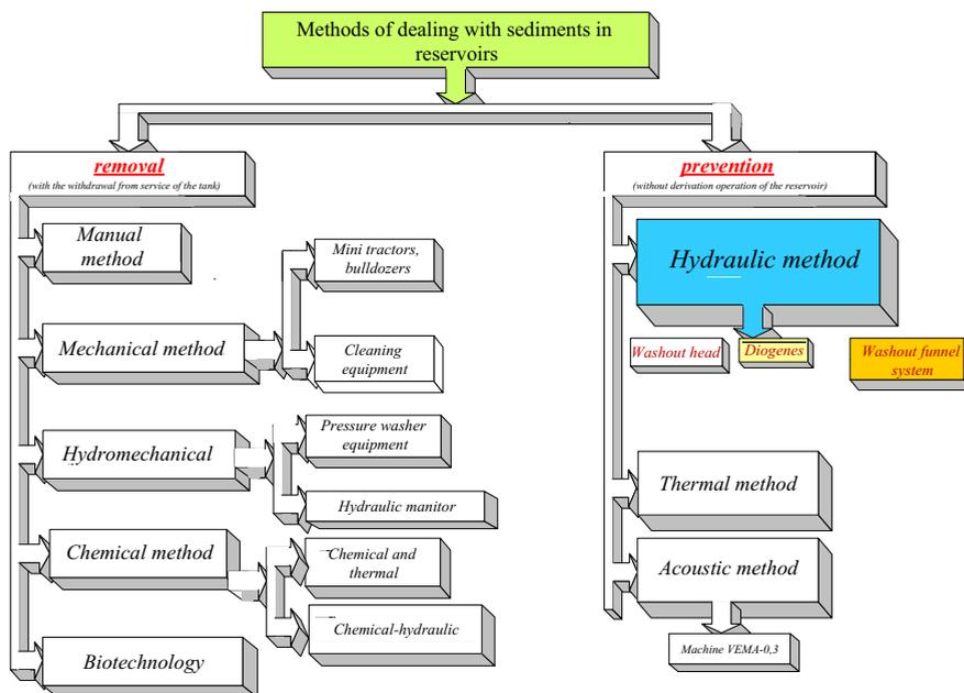
**Fig. 1.** Methods of tank bottoms generation reduction.
