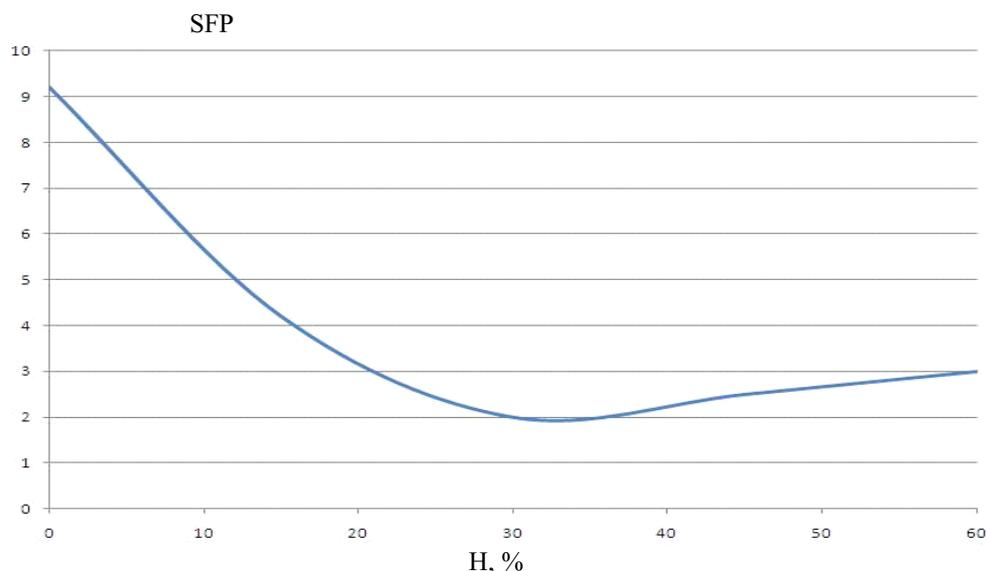
**Fig. 1.** Cement composite SFP vs. nano-modifier content (H).
