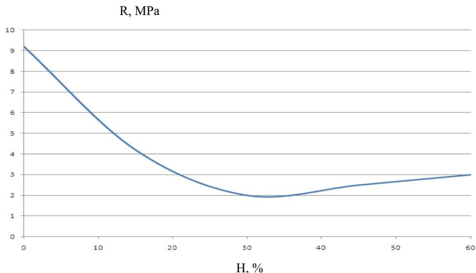
**Fig. 2.** Cement composite strength ( $R$ ) vs. nano-modifier content ( $H$ ).
