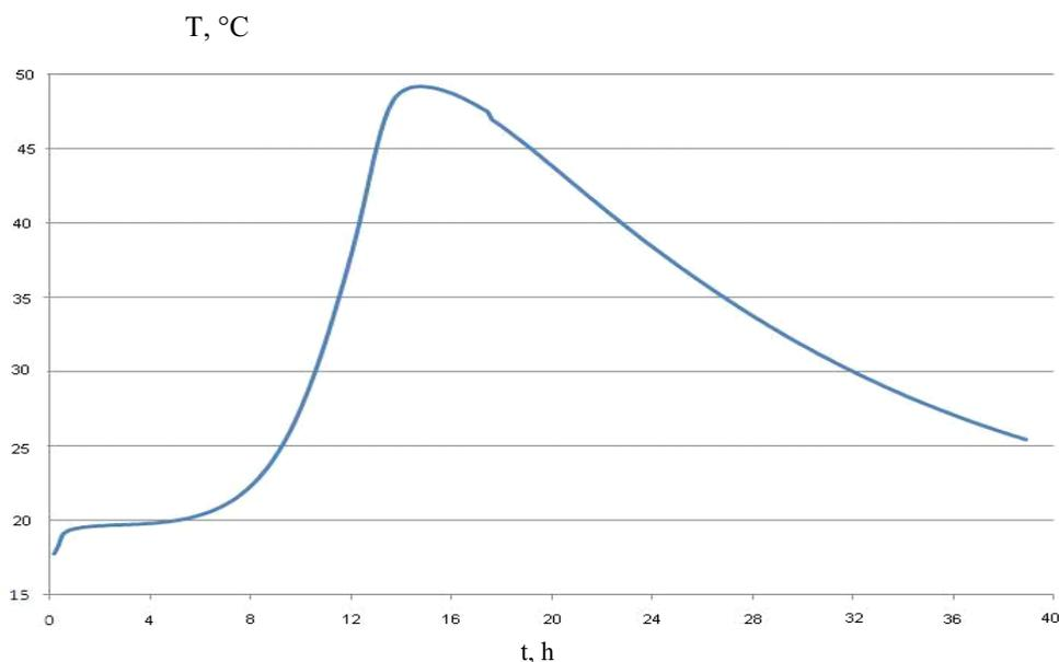
**Fig. 3.** Temperature ( $T$ ) of the cement composite with nano-modifier ( $H$ ) vs. time from the moment of mixing.
