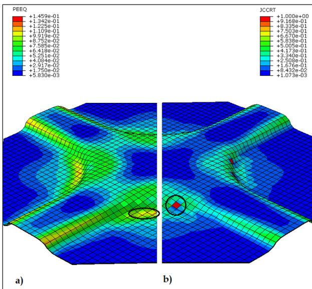
**Figure 8.** Obtained results using the identified parameters of Johnson-Cook damage model. a) Equivalent plastic strain; b) Damage contour prediction.
