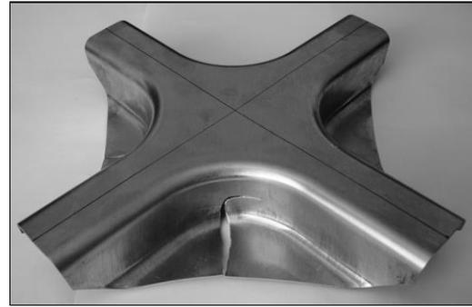
**Figure 5.** Cross-shaped component with breakage.
