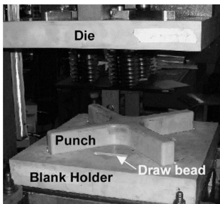
**Figure 4.** Tool geometry and active parts. The punch cross geometry has 487 mm length.
