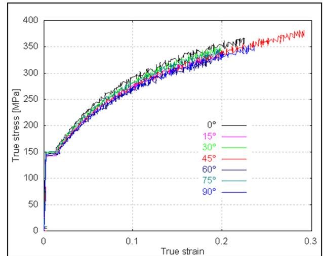
**Figure 1.** Flow stress-strain curve obtained from uniaxial tensile test for AA5182-O, according to different directions relative to the rolling direction [8].
