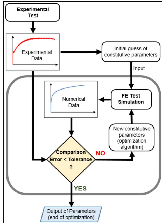
**Figure 3.** Methodology used for the identification of the damage parameters.
