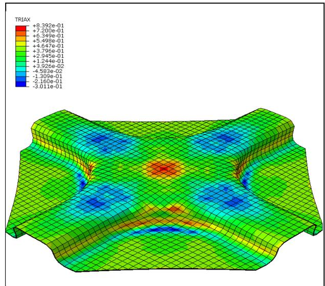
**Figure 9.** Triaxiality levels present in cross-shaped component.
