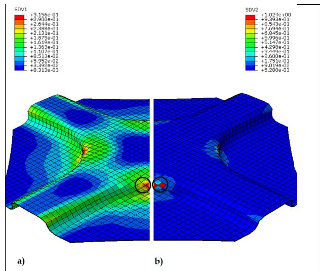
**Figure 6.** Obtained results using the identified parameters of Lemaitre damage model. a) Equivalent plastic strain; b) Damage contour prediction.
