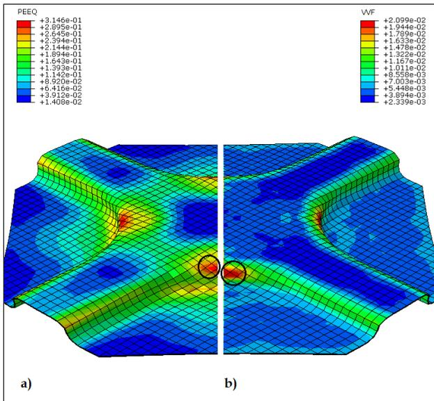
**Figure 7.** Obtained results using the identified parameters of GTN damage model. a) Equivalent plastic strain; b) Damage contour prediction.
