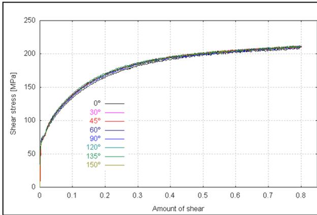
**Figure 2.** Flow curve obtained from monotonic simple shear test for AA5182-O, according to different directions relative to the rolling direction [8].
