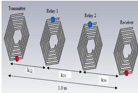
**Fig. 9.** The WPT system with 2 relay coils.
