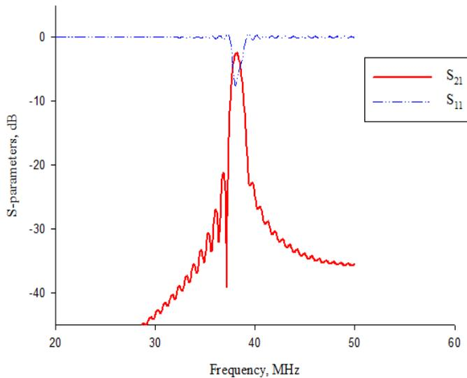
**Fig. 10.** Simulation results of  $S_{11}$  and  $S_{21}$  parameters when inserting 2 relay coils.
