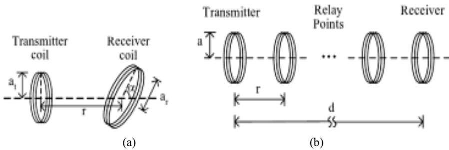
**Fig. 1.** (a) The typical WPT system and (b) WPT with relay coils.
