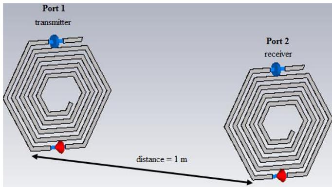
**Fig. 3.** Transmitter and receiver coils of atypical WPT system.
