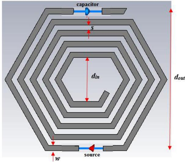
**Fig. 2.** Layout for LC resonator.
