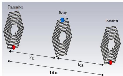
**Fig. 5.** WPT system with a relay coil.
