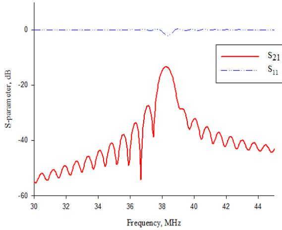
**Fig. 6.** Simulation results of  $S_{11}$  and  $S_{21}$  parameters with a relay coil.
