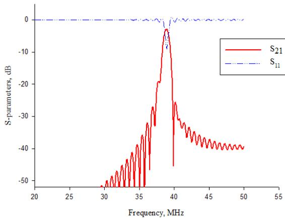
**Fig. 8.** Simulation results of  $S_{11}$  and  $S_{21}$  parameters when relay is biased to the transmitter.
