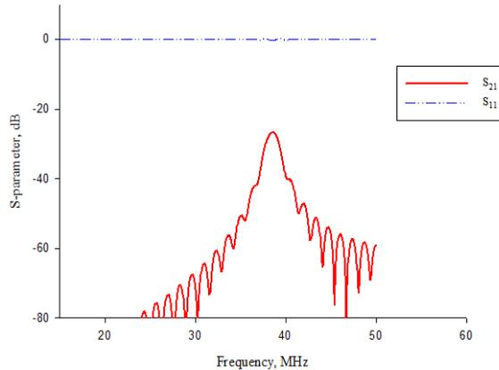
**Fig. 4.** Simulation results of  $S_{11}$  and  $S_{21}$  for a typical WPT system.
