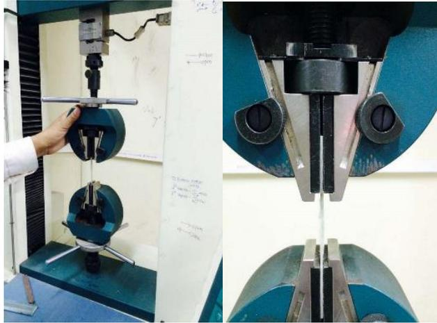
**Fig. 2.** Tensile test on the UTM machine.
