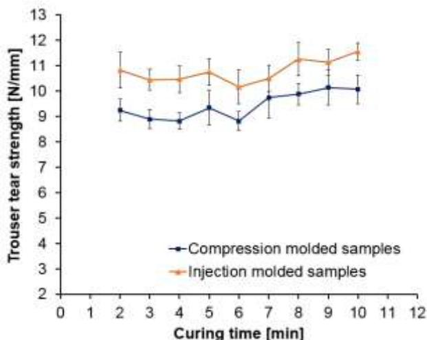
Figure 9. Trouser tear strength vs. curing time
