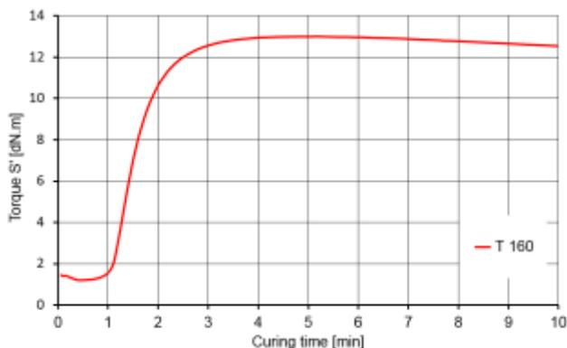
**Figure 1.** Curing curve for 160 °C
