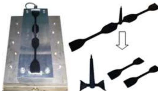
**Figure 3.** Production of testing samples by injection molding
