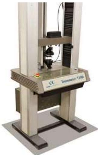
**Figure 5.** Tensile stress machine Tensometer 2000
