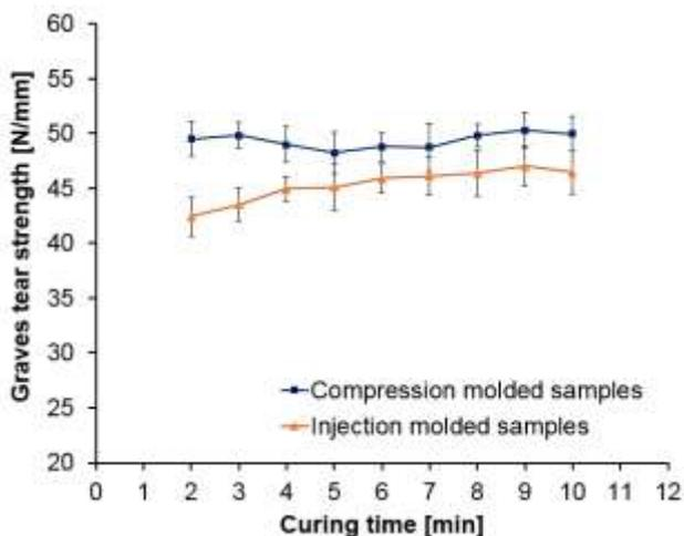
Figure 7. Graves tear strength vs. curing time
