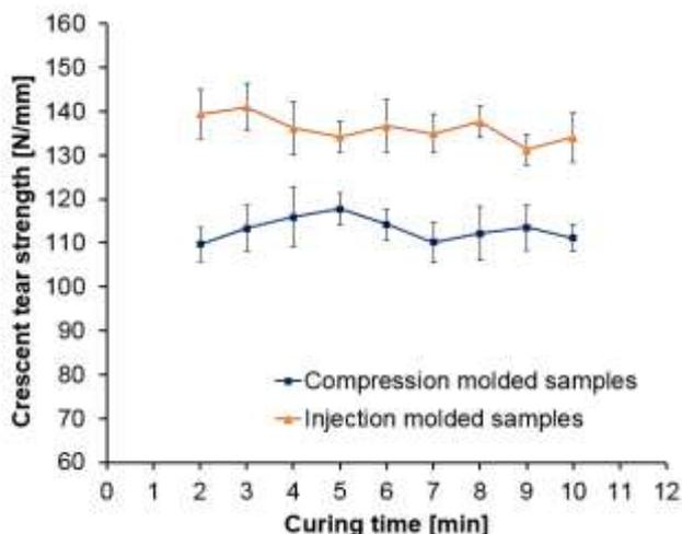
Figure 8. Crescent tear strength vs. curing time
