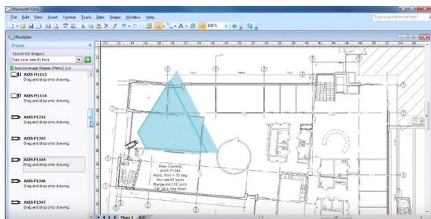
Figure 6. Example of CCTVs installation in Microsoft Visio [6]
