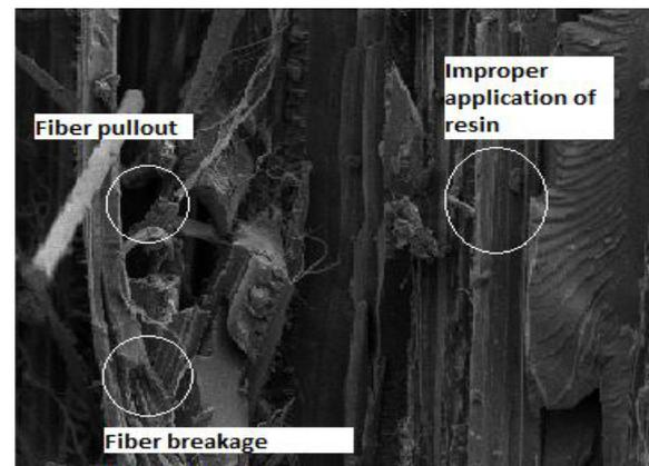
Figure 5. Double shear test SEM image
