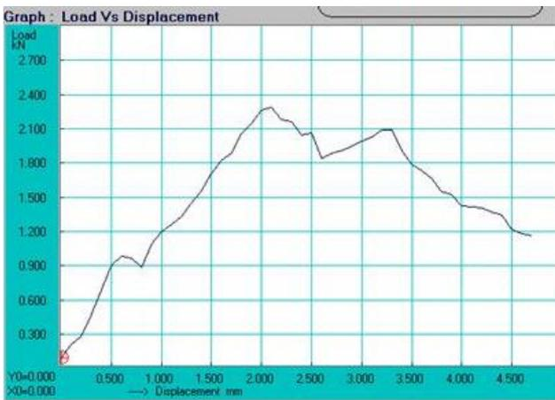
Figure 4. Double shear test graph (composite III)
