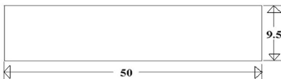
**Figure 1: Double shear test specimen [ASTM: D5379]**
