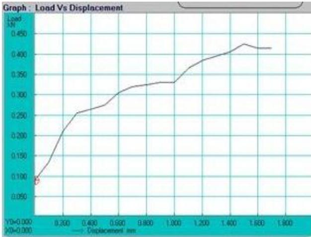
Figure 3. Double Shear Test Graph – (Composite II)
