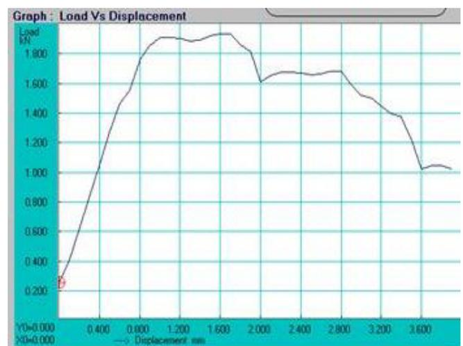
**Figure 2. Double Shear Test Graph- (Composite I)**
