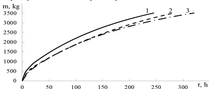
**Fig. 4.** Dynamics of 1 m<sup>3</sup> tank filling ( $t_{CaCl} = -20^{\circ}C$ ): 1 – flat ends of the tank walls, 2 – ellipticity of the bottom wall, 3 – ellipticity of the two end tank walls.
