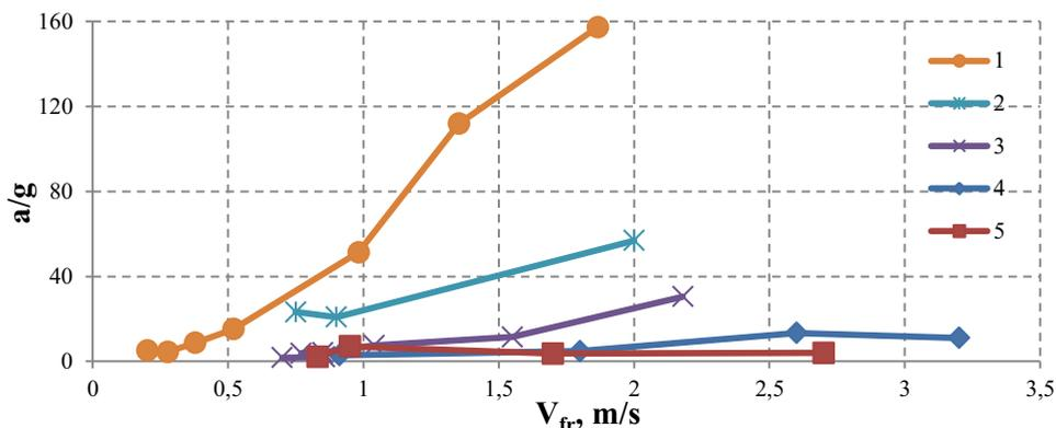
**Fig. 5.** Amplitude acceleration of the interface vs. average velocity. 1 – pure R21; 2 – R21 + 0.0077% SiO<sub>2</sub> in a day after nanoparticles addition; 3 – R21 + 0.0077% SiO<sub>2</sub> in two days; 4 – R21 + 0.0077% SiO<sub>2</sub> in nine days (series 1); 5 – R21 + 0.0077% SiO<sub>2</sub> in nine days (series 2).
