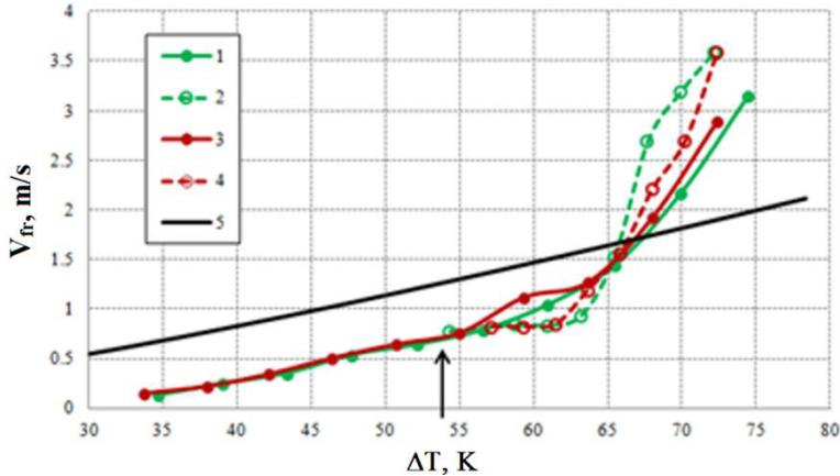
**Fig. 2.** Average front velocity vs. wall superheat. 1 – heater No.1, pure R21; 2 – heater No.1, R21 + 0.0077% SiO<sub>2</sub>; 3 – heater No.2, pure R21; 4 – heater No. 2, R21 + 0.0077% SiO<sub>2</sub>; 5 – calculation by model [5]. The arrow indicates the minimal value of overheating, when the evaporation front is initiated in nanofluid.
