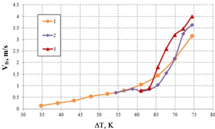
**Fig. 3.** Front velocity vs. wall superheat on heater No. 1 in different experimental series. 1 – pure R21; 2 – R21 + 0.0077% SiO<sub>2</sub> in two days nanoparticles addition; 3 - R21 + 0.0077% SiO<sub>2</sub> in nine days.
