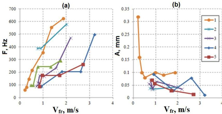
**Fig. 4.** (a) – frequencies and (b) – amplitudes of fluctuations of the front interface on heater No. 1 depending on average velocity. 1 – pure R21; 2 – R21 + 0.0077%  $\text{SiO}_2$  in a day after nanoparticles addition; 3 – R21 + 0.0077%  $\text{SiO}_2$  in two days; 4 – R21 + 0.0077%  $\text{SiO}_2$  in nine days (series 1); R21 + 0.0077%  $\text{SiO}_2$  in nine days (series 2).
