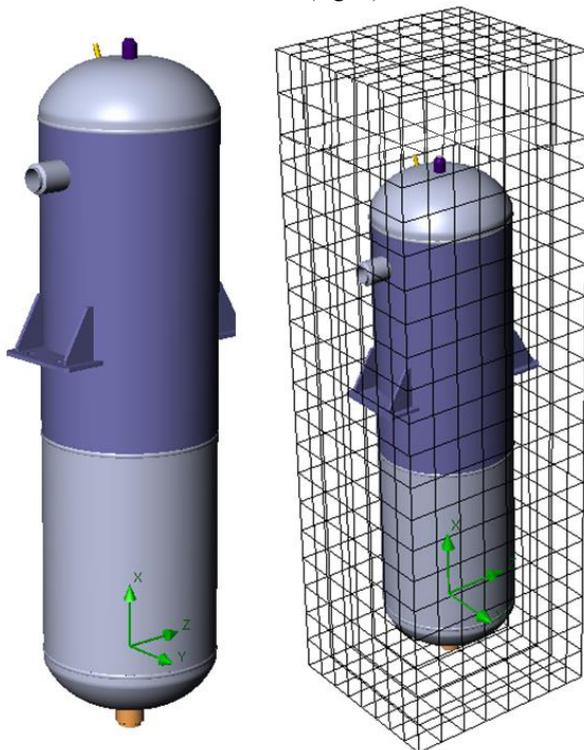
**Fig. 1.** Three-dimensional structure of the degasser and the basic grid of the model.
