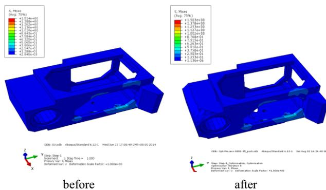
Figure 4. The comparison of stress of outer wheel holder before and after optimization design.
