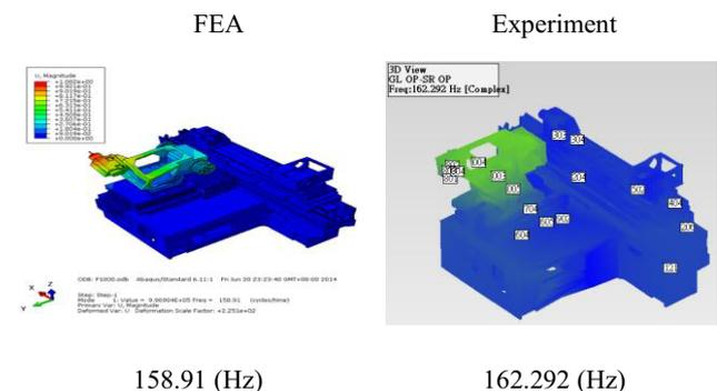
Figure 2. CNC grinding mechanical structure.
