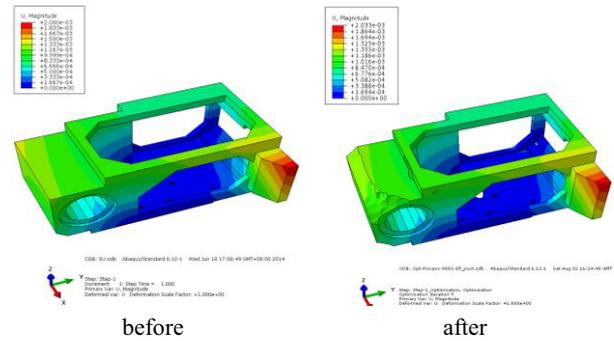
Figure 5. The comparison of displacement of outer wheel holder before and after optimization design.
