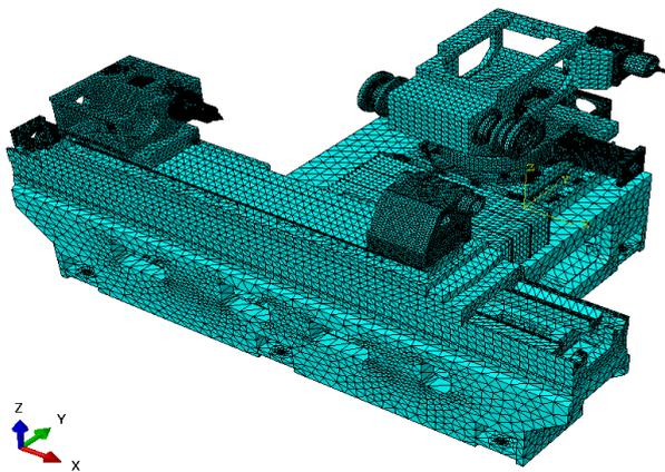
Figure 1. CNC grinding mechanical structure.
