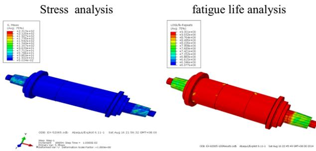
Figure 3. Fatigue analysis of spindle.
