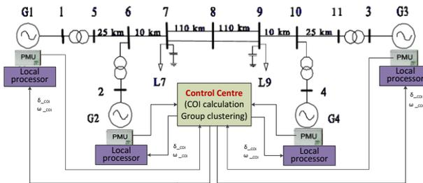
Figure 3. Two-area four-machine power system
