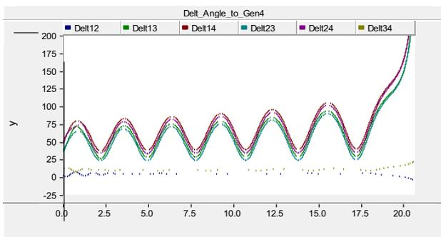
Figure 4. Rotor angle between the generators
