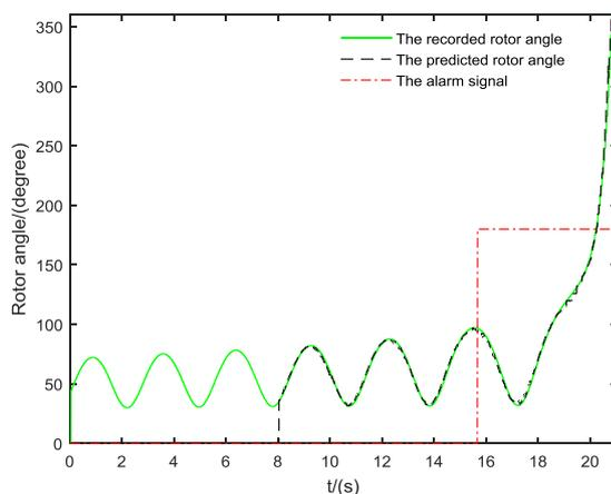
Figure 5. Predicted rotor angle via improved Prony algorithm.
