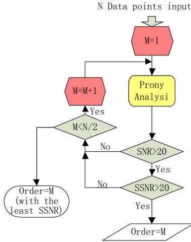
Figure 2. The order determination procedure
