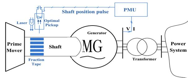
Figure 1. Rotor angle measurement
