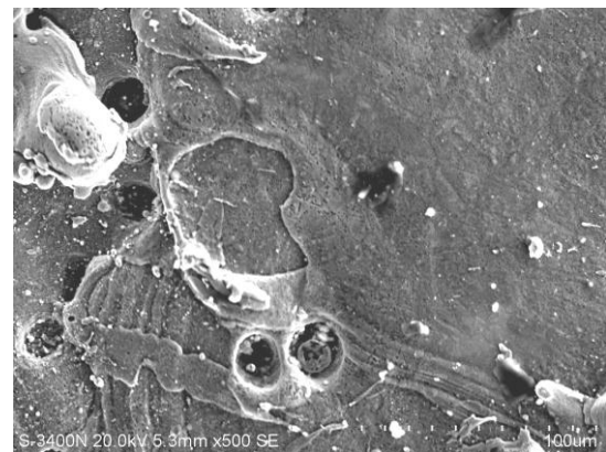
Figure 1. SEM image of EDMed surface machined on SS400 with (a) copper and (b) graphite electrode.
