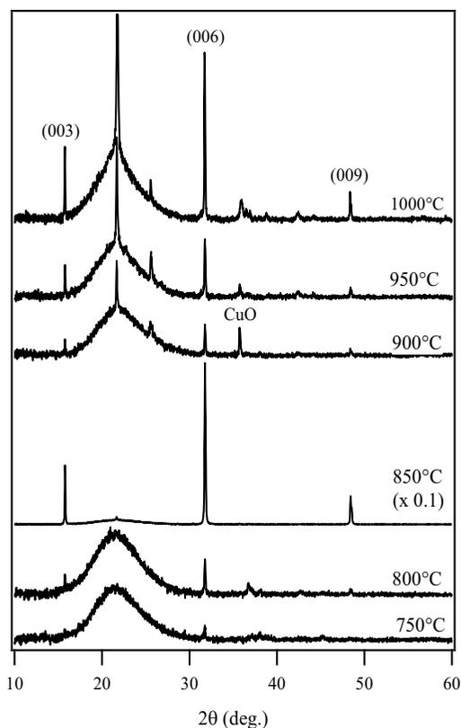
Fig. 1. XRD patterns of the films annealed at 750 -1000°C.
