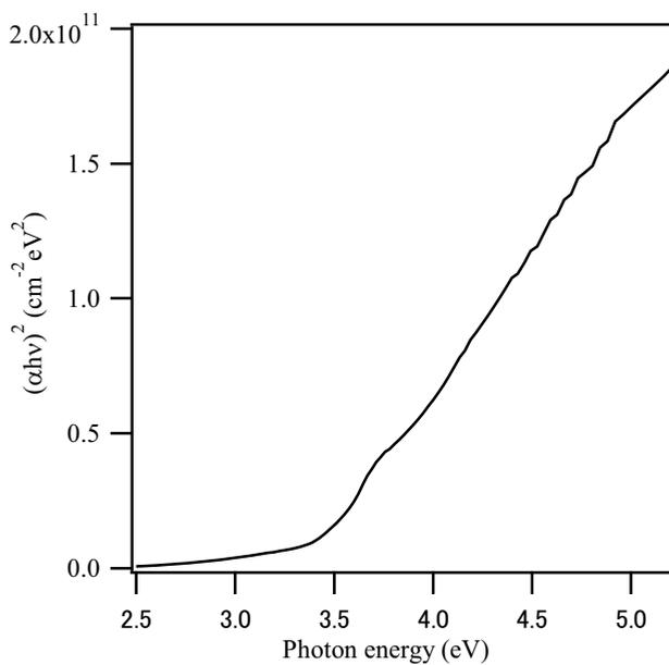
**Fig. 3.** Tauc plot of the film annealed at 850°C
