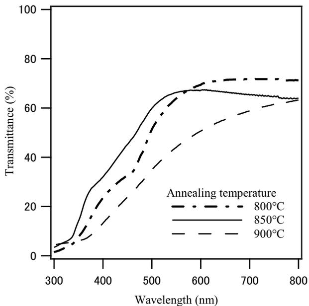
**Fig. 2.** Transmission spectra of the annealed films.
