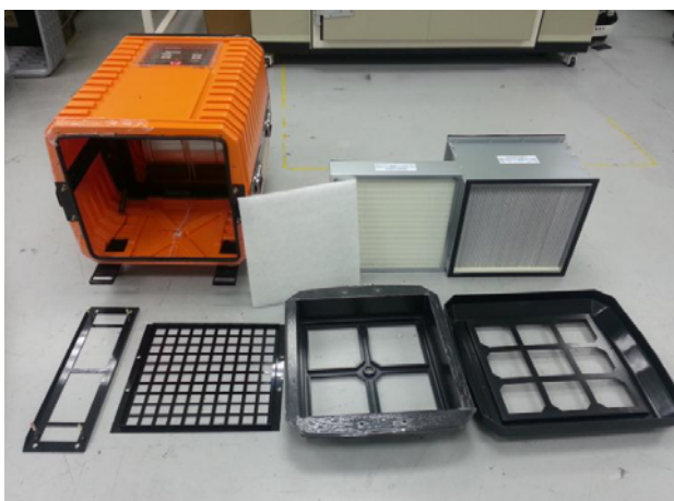
Figure 1. Commercial sound pressure machine for removing asbestos.
