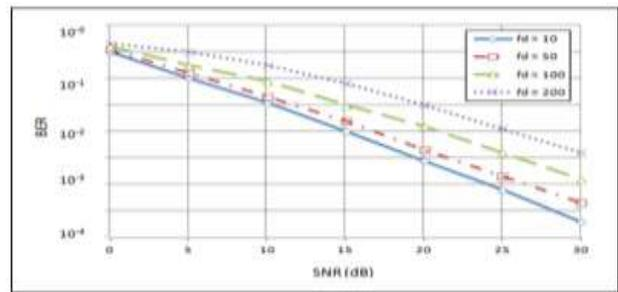
**Figure. 3.** The BER performance vs. SNR, with time-orthogonal transmitted training sequences (Scheme I)
