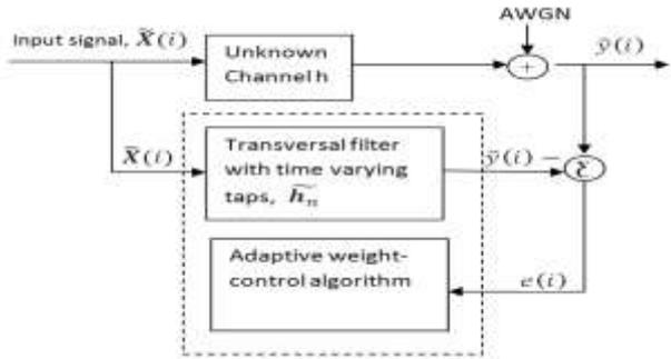
**Figure 1.** Illustration of adaptive filter modelling of unknown channel.
