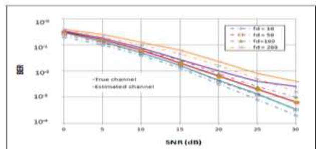
**Figure. 5.** The BER performance vs. SNR, with simultaneously transmitted training sequences (Scheme II)
