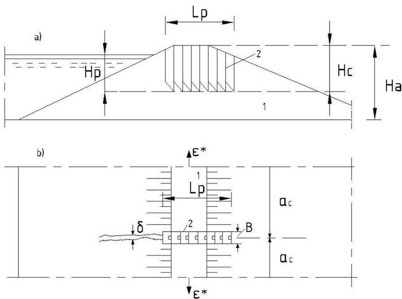
**Figure 2.** Transverse rows of pile
