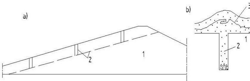
**Figure 1.a** Homogeneous dam of cohesive soil
