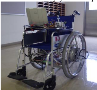
(a) Developed electric-wheelchair
