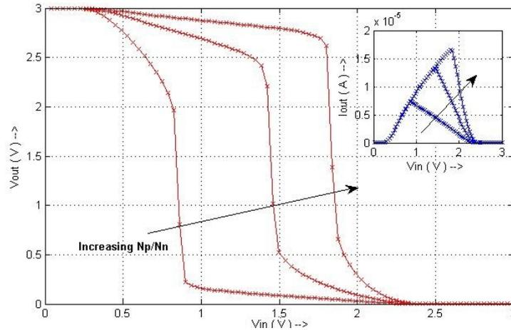
Figure 6. Transfer and current characteristics with different ( $N_p/N_n$ ) and  $V_{dd}=3V$ .
