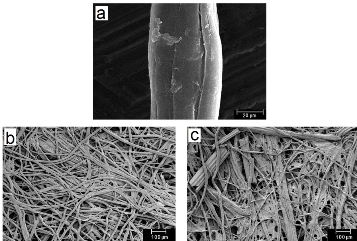
**Figure 2.** SEM images of a)KF-PANI b)neat KF sheet c) KF/25KF-PANI
