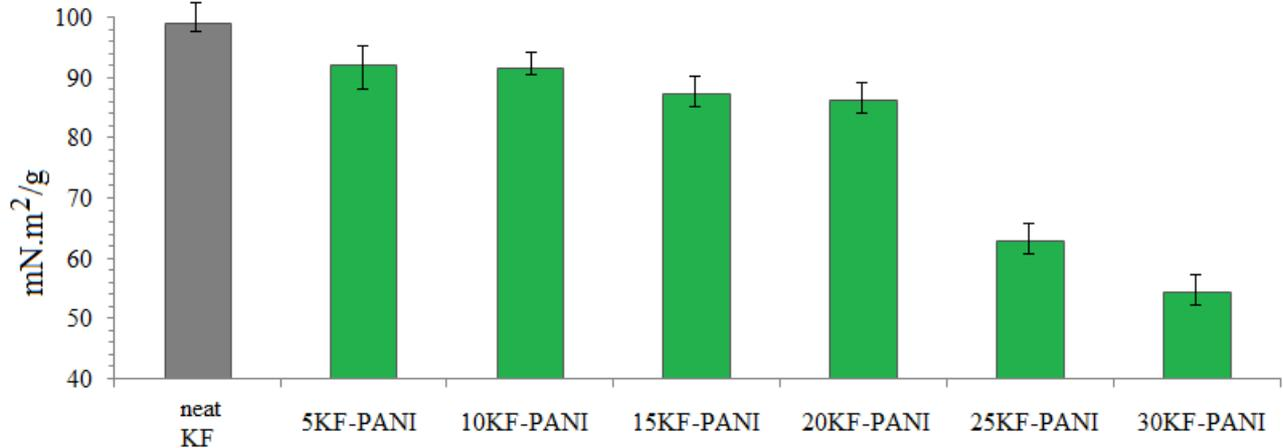
**Figure 1.** Tear index of KF sheets modified with KF-PANI.
