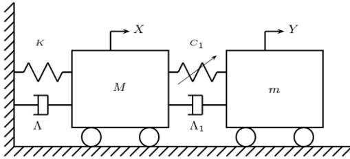
**Figure 1.** Scheme of the studied system, 1<sup>st</sup> cable mode coupled with a NES.
