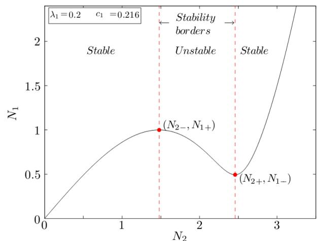
**Figure 2.** Invariant manifold in fast time for  $c_1 = 0.216$  and  $\lambda_1 = 0.2$
