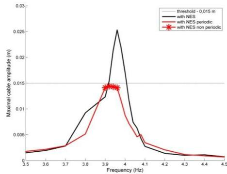
**Figure 6.** Result Frequency response of the cable with and without coupled NES. The cable is excited by external periodic force with the frequency in the vicinity if the first mode and the NES threshold.
