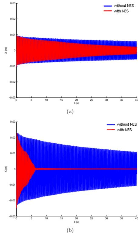
**Figure 4.** Experimental results comparing test with and without NES for a step release test (a) under the threshold and (b) above the threshold
