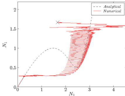
**Figure 3.** Theoretical invariant manifold of the dimensionless system versus the results obtained from numerical integration of general system equations for a free response with efficient NES design.
