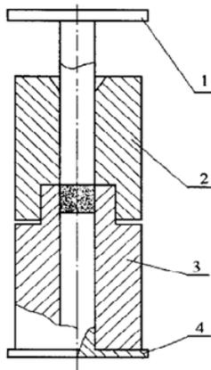
**Figure 1.** The apparatus for compacting and extruding the material
