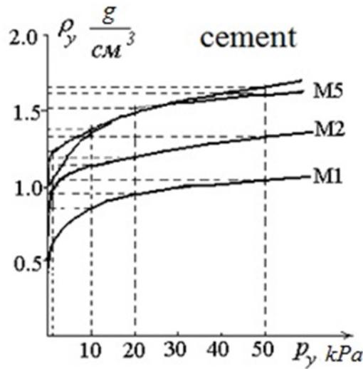
**Figure 2.** Density powders according to the pressure
