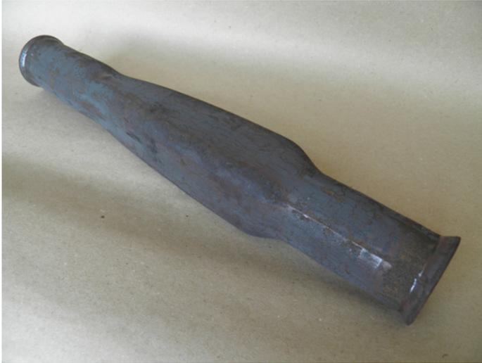
**Figure 1.** Final product of internal high pressure forming and subsequent Q&P processing.
