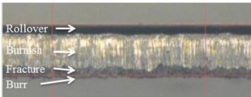
**Figure 4.** Cross-section of shearing experiment.
