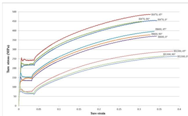
**Figure 1.** Flow stresses of plate materials.
