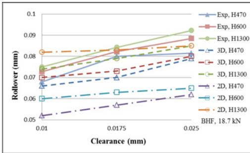
**Figure 11.** Variation of rollover with clearance.
