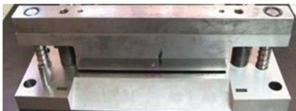
**Figure 2.** Assembly of punch and die of shearing experiment.
