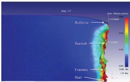
**Figure 6.** Side-view of 3-D simulation.
