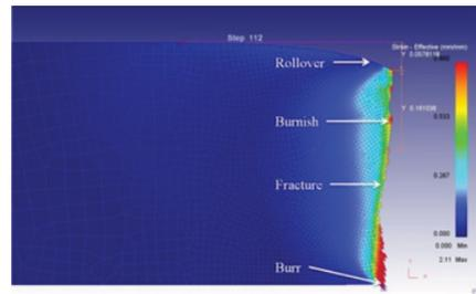
**Figure 7.** Side-view of 2-D simulation.
