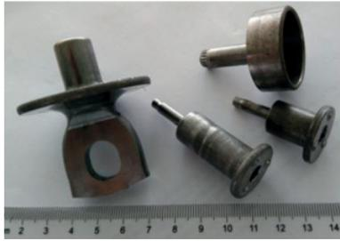
**Figure 3.** Cold formed Parts with large deformation (provided by Ritai).
