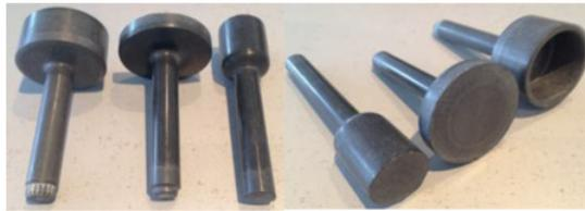
**Figure 4.** Cold formed Parts with extreme localized forward, upset and backward extrusion.
