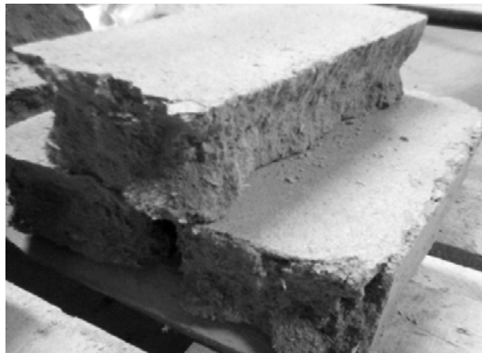
Figure 5: Crushed brick after Compressive Strength Test
