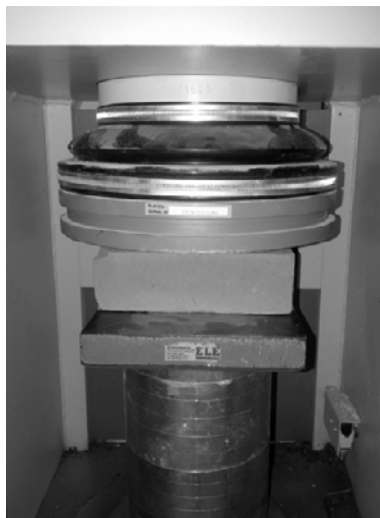
Figure 1: Compressive Strength Test for Brick
