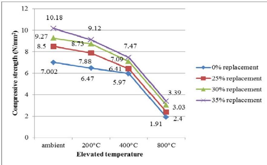
Figure 6: Effect of elevated temperature to the residual compressive strength of cylinder samples
