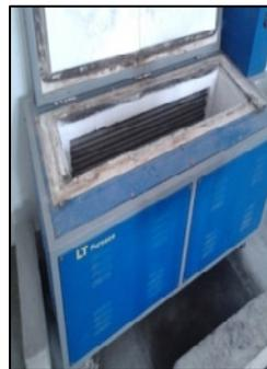
Figure 2: Electric furnace
