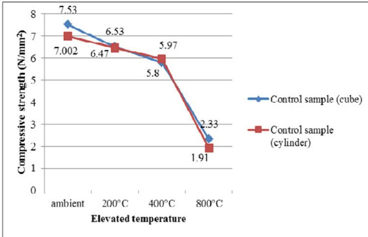
Figure 4: Effect of elevated temperature to the compressive strength of controlled samples
