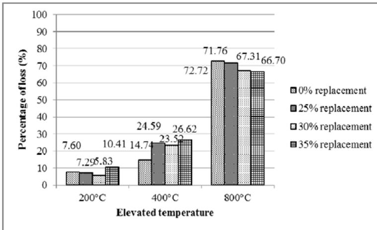
Figure 8: Percentage of compressive strength loss due to elevated temperature (cylinders)
