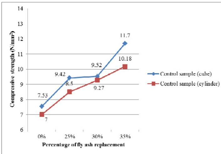
Figure 3: Effect of fly ash to the compressive strength of controlled samples
