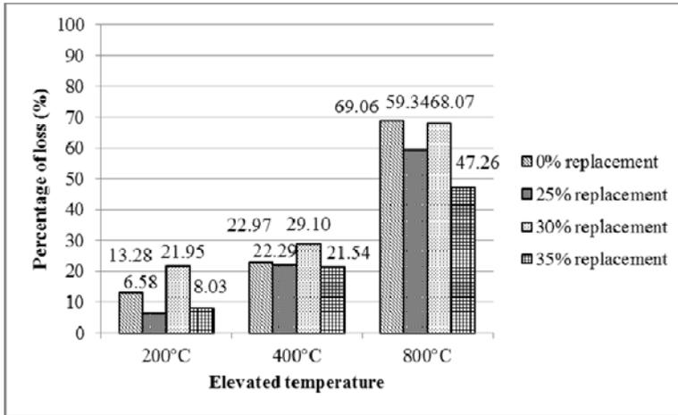
Figure 7: Percentage of compressive strength loss due to elevated temperature (cubes)
