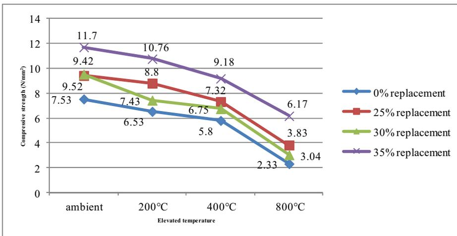
Figure 5: Effect of elevated temperature to the residual compressive strength of cube samples
