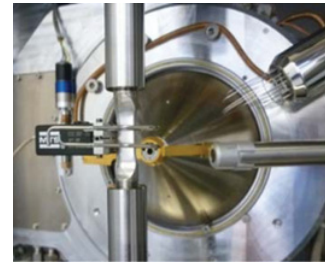
Figure 3. Specimen mounted in the servo-hydraulic test rig of the large chamber SEM at the ZMP Fürth.
