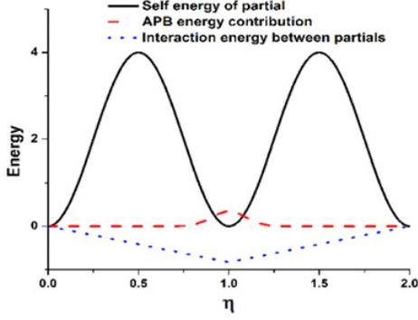
**Figure 1.** Variation of the various components of  $E_o$  with  $\eta$  for a pair of straight dislocations.
