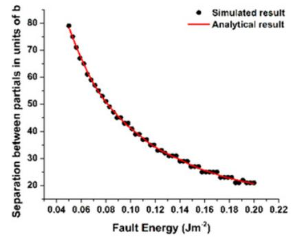
**Figure 4.** A comparison between simulated and analytically-solved values of separation between partial dislocations as a function of fault energy.
