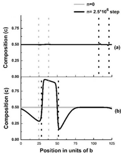
**Figure 8.** Concentration profile across the extended superdislocation at different times for (a)  $M_r = 0.1$ , (b)  $M_r = 10$  for  $\text{Co}_3(\text{Al,W})$  system. Dotted vertical lines represent the position of superpartial dislocations and solid lines indicates the composition profile across the slip plane.
