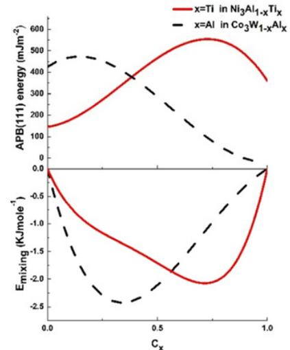
**Figure 5.** Composition dependence of APB energy and enthalpy of mixing in  $Ni_3Al(Ta/Ti)$  and  $Co_3W(Al)$ .
