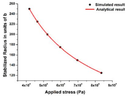
**Figure 3.** A comparison between simulated and analytically-solved values of radius of stable loop as a function of stress.
