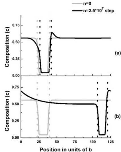
**Figure 7.** Concentration profile across the extended superdislocation at different times for (a)  $M_r = 0.1$ , (b)  $M_r = 10$  for  $\text{Ni}_3(\text{Al,Ti})$  system. Dotted vertical lines represent the position of superpartial dislocations and solid lines indicates the composition profile across the slip plane.
