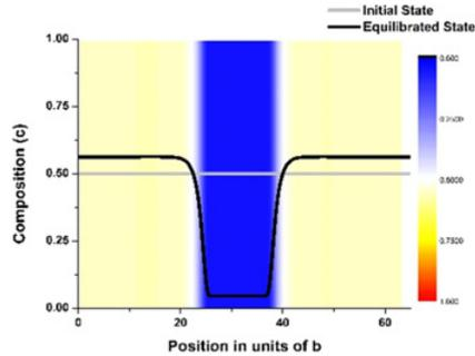
**Figure 6.** The initial and equilibrated concentration profiles in  $\text{Ni}_3\text{Al}_{1-c}\text{Ti}_c$  alloy are superimposed on top of the composition map. The deep blue shades correspond to a low Ti concentration.
