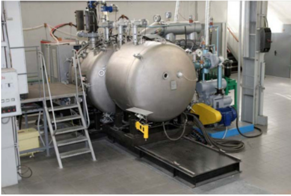
Figure 1. Industrial-scale high-gradient plant with the sluice chamber UVNS-6.
