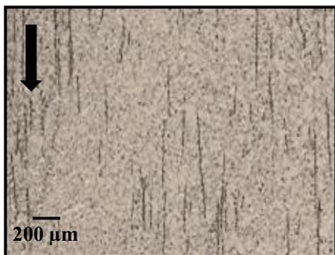
**Figure 4:** Aligned fibers at S2 skin obtained for F-5 moldings
