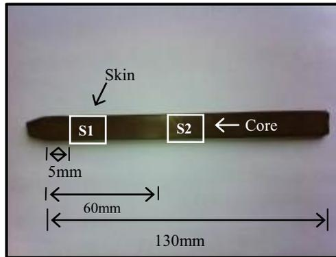
**Figure. 1** Positions of samples for fiber orientation analysis shown on a green molding
