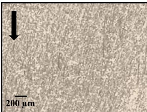
**Figure 2:** Aligned fibers at S1 skin obtained for F-5 moldings
