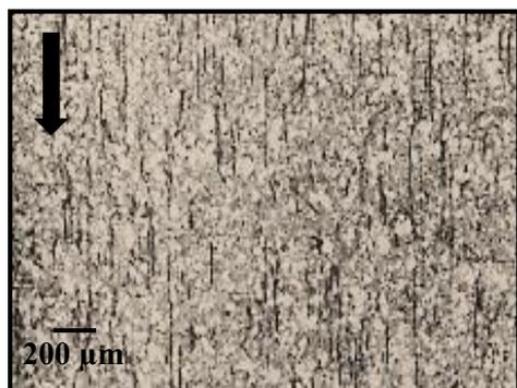
**Figure 8:** Aligned fibers at S2 skin attained for F-10 moldings
