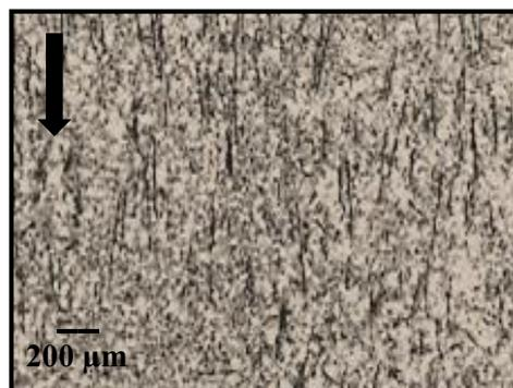
**Figure 9:** Aligned fibers attained at S2 core for F-10 moldings
