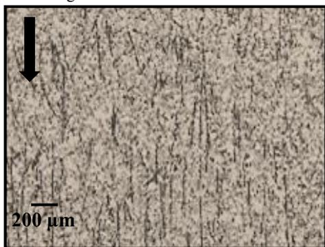
**Figure 6:** Aligned fibers at S1 skin obtained for F-10 moldings
