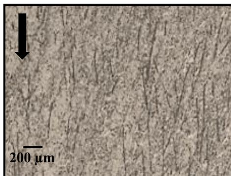
**Figure 5:** Aligned fibers at S2 core attained for F-5 moldings
