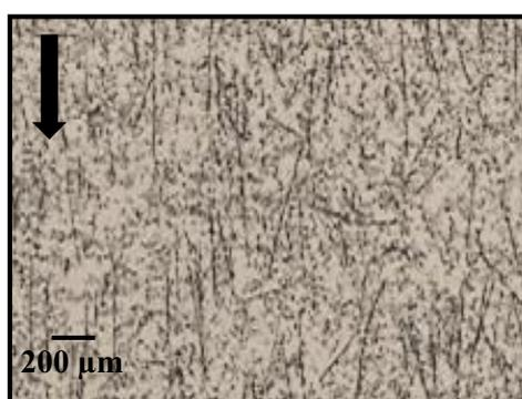
**Figure 7:** Partially aligned fibers at S1 core obtained for F-10 moldings
