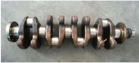
Figure 1. Four-cylinder four stroke engine crankshaft.
